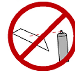
Bad - paint will get under the stencil
